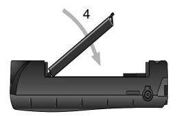
bottom end first, into the compartment, and then press the battery downward until it clicks into place.
