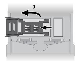
4. Insert the SIM card into the tray with the notch up and the gold plate facing out.
