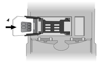
5. Push down the SIM card tray and slide the tray to the right to lock it in place.
